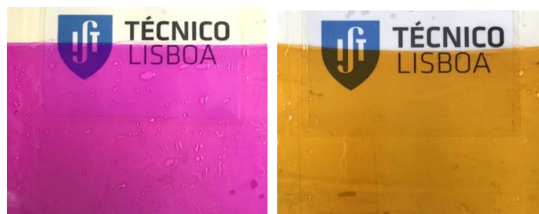
Figure 4: CA99-RB-PURE G4 pink membrane (left) and CA95-SiO 2 -(CH 2 ) 3 NH 2 -MR orange membrane (right).
